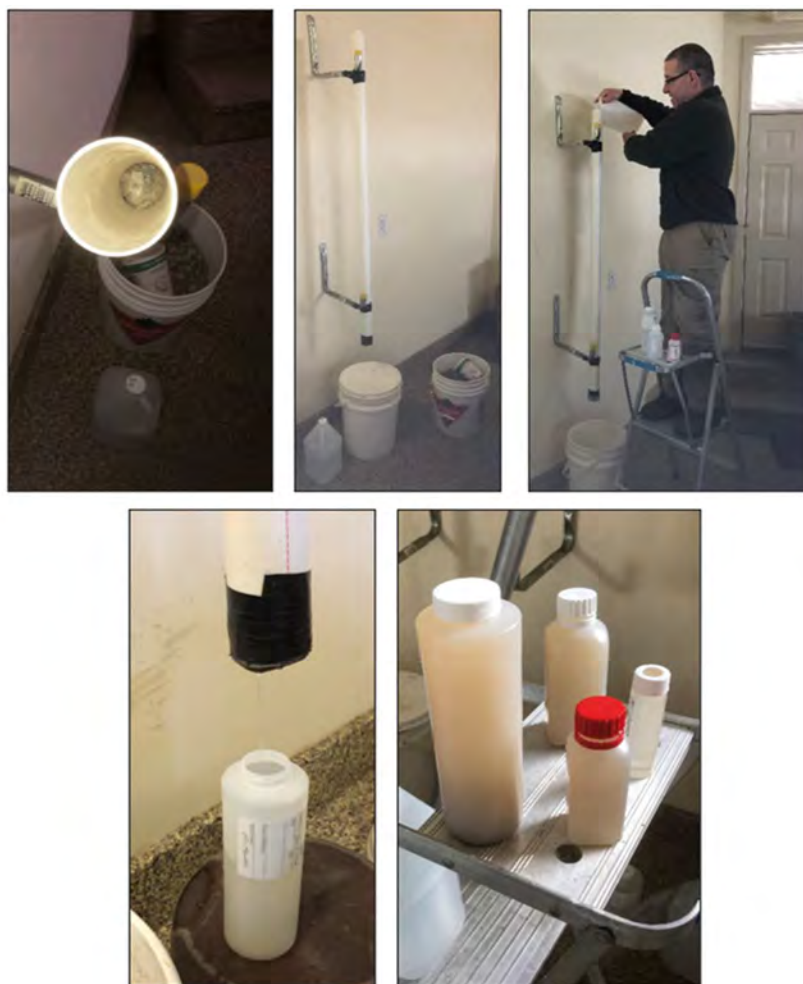
Figure 1. Experimental setup, execution, and sample turbidity noted.
