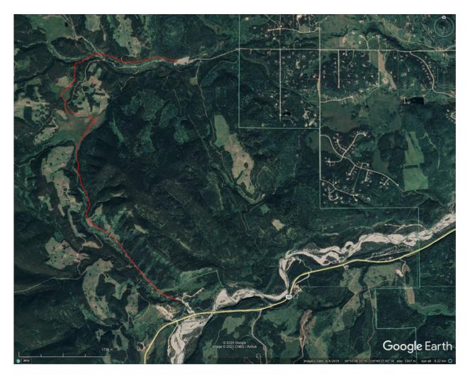
The route shown in the image is approximately 8.75 km and, at a conceptual level, suggests a road could be constructed for less than \$10 million. The conceptual route selected limits gradients to a maximum of 8% and we have provided in a second image on the following page which shows the road profile on an exaggerated vertical scale; this demonstrates, at a conceptual level, none of these gradients are greater than 8%.
