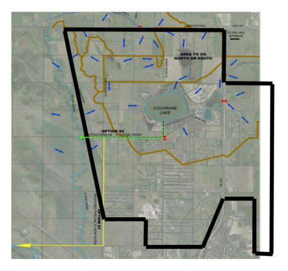
ASP: Black Line Discharge to Horse Creek Yellow - Proposed pipe to Bow River Orange – Catchment area
