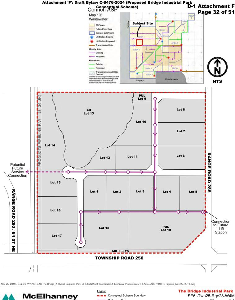
Figure 11 Wastewater Servicing
