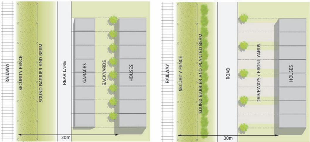
FIGURES 5 (LEFT) & 6 (RIGHT) // SETBACK CONFIGURATION OPTIONS FOR OPTIMUM SITE DESIGN
