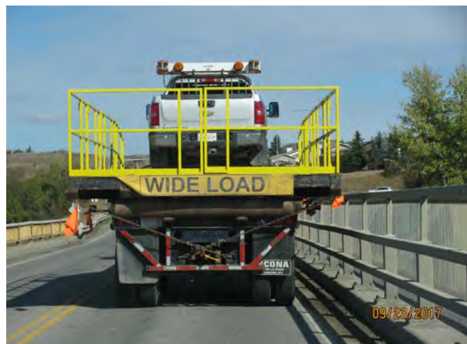
Photo 9: example of overload vehicle crossing a narrow structure on Hwy 22.
