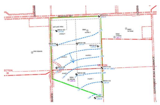
**Figure 3.** Location of monitoring wells and local water wells (used in the 2020 SLR Hydrogeological Assessment) and mapped water table elevations and contours<sup>6</sup>. (Note: blue arrow indicates direction of flow)
